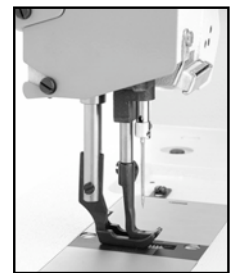
Unison feed assures even feed when sewing multiple layers
