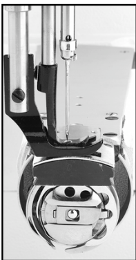
Small bobbin allows sewing around smaller tubular products.
